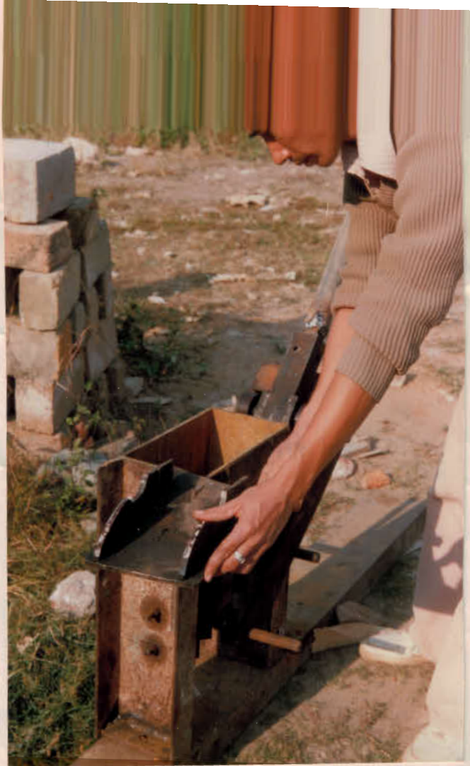
Experimentation with a cinva ram press
