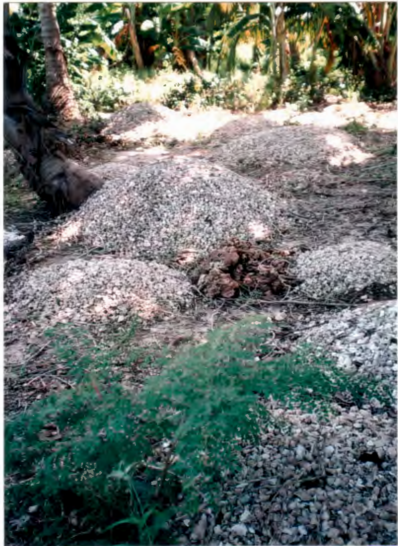
Landbased limestone being broken for aggregate
