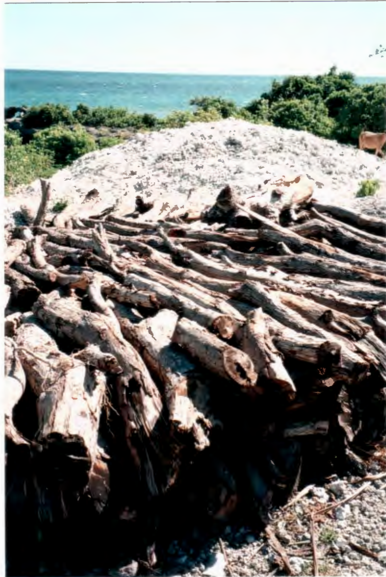
Lime from coral and mangroves for fuel: lime "kiln" on Jibondo
